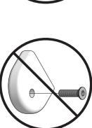
Insert bolts through countersunk hole side of blocks as shown below
