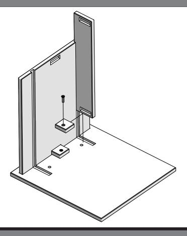
Fit a Brace into the Top's cut out and slide into the small cut out in the Side as shown. Place Square Block (recessed hole side out) into the Brace's cut out, insert a bolt through the block into the Side's threaded hole, and finger tighten.
