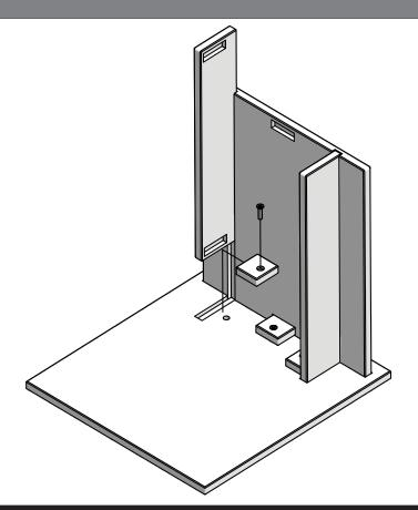
Fit the second Brace into the Top's other cut out and slide into the small cut out in the Side as shown. Place Square Block (recessed hole side out) into the Brace's cut out, insert a bolt through the block into the Side's threaded hole, and finger tighten.
