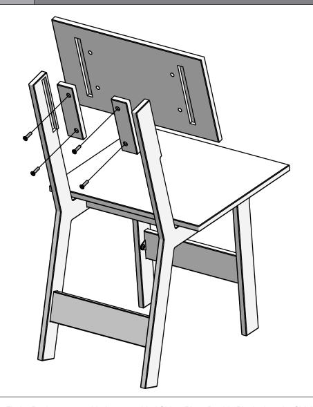
Fit the Seat cut outs with the assembled Sides and Seat Braces. Place Micro Blocks into the Seat Brace pocket cut outs, insert 1/2" Round Head Bolts through the blocks into the Seats threaded holes, and finger tighten.
