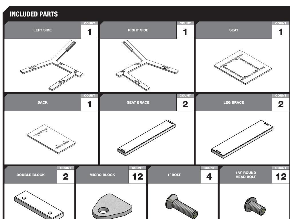
\* It is very important that you finger tighten all bolts into inserts to ensure that you do not cross-thread bolts and inserts before tightening. It will also be easier if you wait to tighten bolts until you have all bolts installed and the piece completely assembled. This will allow for more movement of individual pieces and help in aligning holes with inserts. Use the Allen Tool provided to finish tighten bolt until snug.
