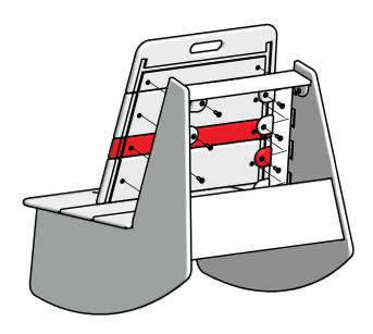
Layout the Back Set so that the groove track cut outs line up. Place Back Set individually over assembled chair sides (start with A then B, C, D) by fitting the groove track cut outs with the Sides and Front Plate. Place G Blocks into the Sides pocket cut outs, insert bolts through the blocks into the Back Sets threaded holes, and finger tighten.
