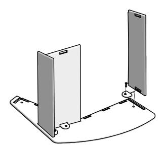
Fit Face Plate short edge into the Left Side's pocket cut out. Place G Block into the Face Plate's pocket cut out, insert a bolt through the block into the Left Side's threaded hole, and finger tighten.
