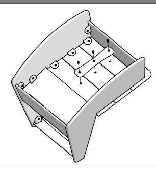
Align Seat Brace holes with the holes of the Seat Set, then insert bolts through the Seat Brace into the Seat Set's threaded holes and finger tighten.
