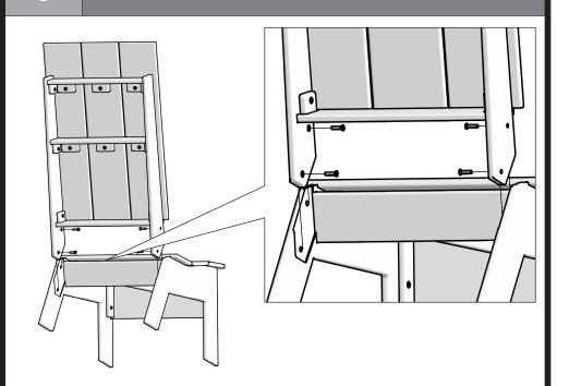
Align Back with seat assembly by fitting Back ends between the Legs. Align the holes in the back with threaded holes in the Legs and insert bolts. Finger tighten.
