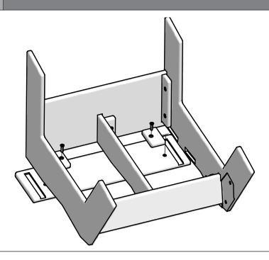
Fit Seat Slat A cut outs with the assembled Legs on Face Plate end. Place Blocks G into Leg cut outs. Insert bolts through the blocks into the seat slat and finger tighten.
