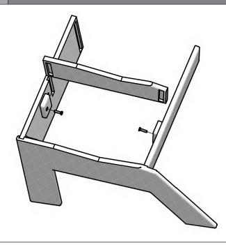
Slide the Seat Brace into cut outs of the Face Plate and Back Brace. Place Blocks G into the Seat Braces cut outs. Insert bolts through the blocks into the threaded holes of the Face Plate and Back Brace and finger tighten.
