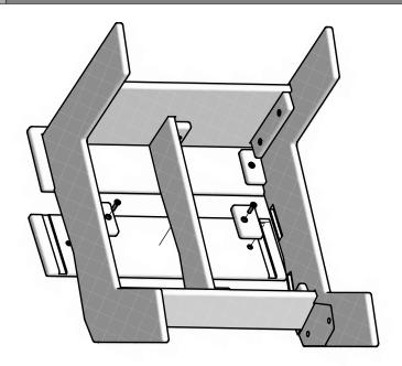
Fit Seat Slat B cut outs with the assembled Legs and align over the middle cut outs in the legs. Place Blocks G into Leg cut outs. Fit Seat Slat B cut outs with the assembled Legs and align over the rear cut outs in the legs. Place Blocks G into Leg cut outs. Insert bolts through the blocks into the seat slats and finger tighten.
