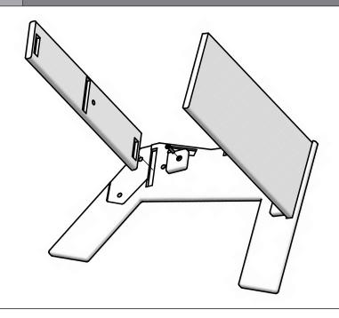
Fit the short edge of the Back Brace with the Left Legs short groove track cut out. Place Block G into the Back Brace cut out. Insert bolts through the block into the Left Legs threaded holes and finger tighten.
