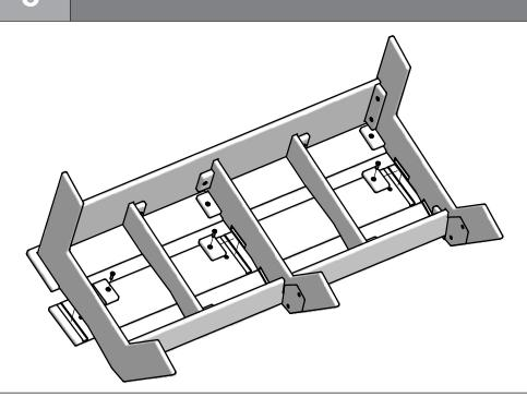
Fit Seat Slat 2 cut outs with the assembled Legs and align over the middle cut outs in the legs. Place Blocks G into the Leg cut outs. Fit the second Seat Slat 2 cut outs with the assembled Legs and align over the rear cut outs in the legs. Place Blocks G into the Leg cut outs. Insert bolts through all the blocks into the seat slats and finger tighten
