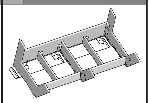
Fit Seat Slat 1 cut outs with the assembled Legs on Face Plate end. Place Blocks G into the Left, Right, and Center Leg cut outs. Insert bolts through the blocks into the seat slat and finger tighten.
