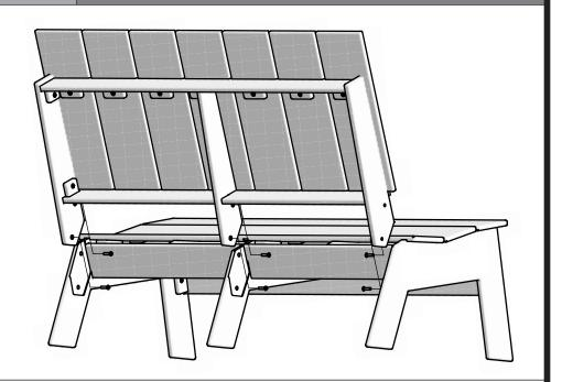
Align Back with seat assembly by fitting Back ends between the legs fitting into notched cut outs of the legs. Align the holes in the back with threaded holes in the Legs and insert bolts. Finger tighten.
