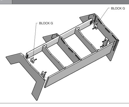
Fit the Left and Right Legs with the ends of the Back and Face Plates. Place Blocks G into the Back Plate cut outs and Blocks B into the Face Plate cut outs. Insert bolts through the blocks into the corresponding plate and finger tighten.
