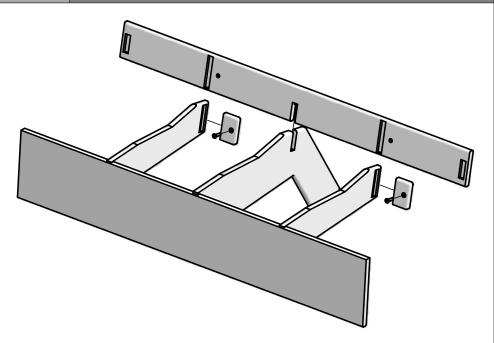
Slide the Back Plate over the Center Leg notched cut out and fit the Seat Brace ends into the Back Plate cut outs. Place Blocks G into the Seat Bracke cut outs and insert bolts through the blocks into the Back Plate and finger tighten.
