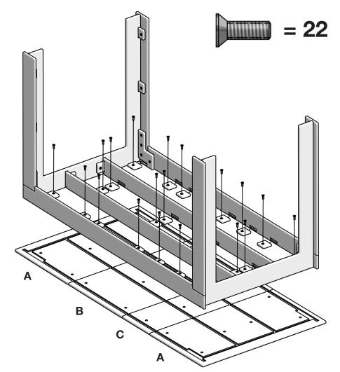
Fit long cut out in Legs with edges of Sides. Legs holes will align with holes in Leg Blocks. Insert bolts through the Leg Block holes into threaded holes of the Leg and tighten.
