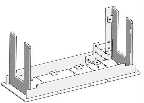
Fit cut out of the Leg with the edge of the Side. Place Square Block into cut out of the Side. Insert a bolt through the block into the Leg's threaded holes and tighten.
