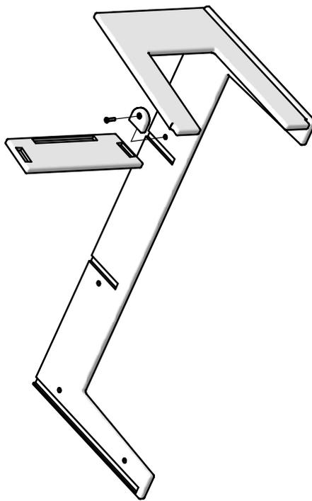
Fit short edge of the Brace into the Side's pocket cut out with the Braces pocket cut out facing the threaded hole in the Side. Place Block G into the Brace's pocket cut out, insert bolts through the block into the Side's threaded holes, and finger tighten.
