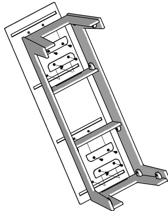
Repeat steps 1&2 to attached remaining side, brace, and end. Fit Top groove track cut outs with assembled Ends and Braces. Place Blocks B into the Brace's and End's pocket cut outs, insert bolts through the blocks into the Tops's threaded holes, and finger tighten. Using provided wrench securely tighten all bolts.
