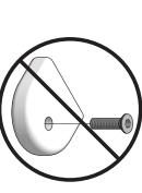
Insert bolts through countersunk hole side of blocks as shown below. **BLOCK & BOLT INSTALLATION**
