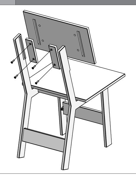
Fit the Back cut outs with the assembled Sides. Place Double Blocks into the Side's pocket cut outs (recessed hole side out), insert 7/8″ Bolts (orange tip) through the blocks into the Seats threaded holes, and finger tighten.
