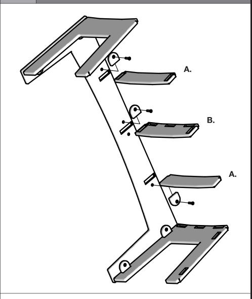
**A.** Fit short edge of the Small Ribs into the Side's outer pocket cut outs with the Ribs pocket cut out facing the threaded hole in the Side. Place Blocks G into the Rib's pocket cut outs, insert bolts through the blocks into the Side's threaded holes, and finger tighten.
