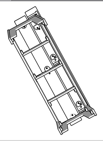
Fit end Seat Slats (A) groove track cut outs over Ends, Small Ribs, and Large Rib(s). Place Blocks G into the Rib's and End's pocket cut outs, insert bolts through the blocks into the Seat Slat's threaded holes, and finger tighten.
