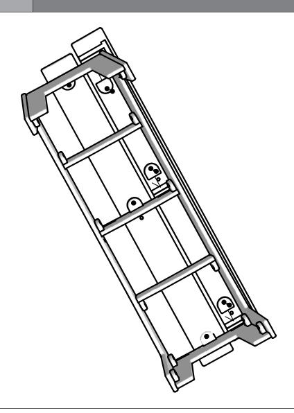
Fit end Seat Slats (A) groove track cut outs over Ends, Small Ribs, and Large Rib(s). Place Blocks G into the Rib's and End's pocket cut outs, insert bolts through the blocks into the Seat Slat's threaded holes, and finger tighten.
