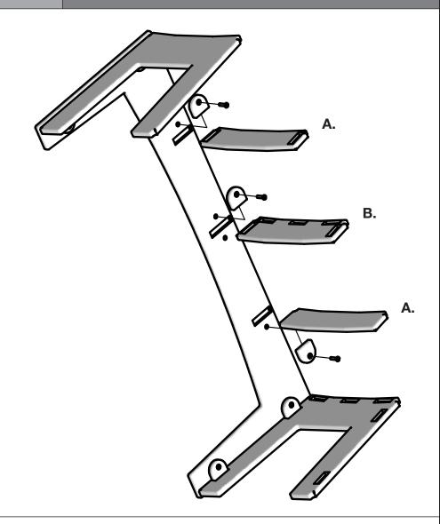
**A.** Fit short edge of the Small Ribs into the Side's outer pocket cut outs with the Ribs pocket cut out facing the threaded hole in the Side. Place Blocks G into the Rib's pocket cut outs, insert bolts through the blocks into the Side's threaded holes, and finger tighten.
