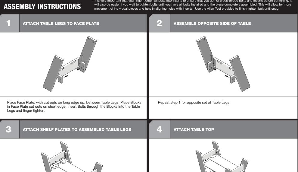
Place Shelf Plates next to each other and align the groove track cut outs with the Face Plates of already assembled Legs. Place Blocks into Face Plate cut outs and insert Bolts through the Blocks and finger tighten.
