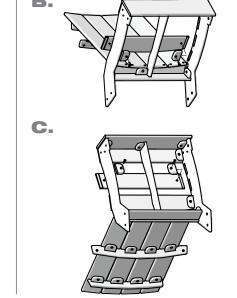
A. Fit groove track cut outs of front Seat Slat with assembled chair base frame. Place Block G's in Base Side's, insert bolts, and finger tighten.
