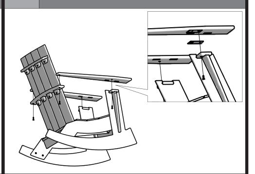
Place Bottle Opener (protective film side out) into the Right Arm's cut out then remove film, place the Arms on top of the Legs and middle support of the Back. Align Leg and support holes with corresponding Arm holes. Insert bolts into the Arms and finger tighten.
