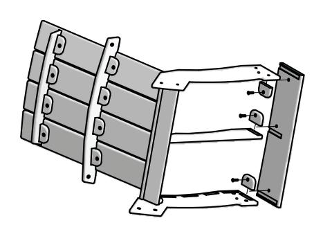
Align Face Plate cutouts with ends of corresponding Base Sides and Seat Support. Place Block G's into Base Side and Seat Support cutouts. Insert Bolts through the Block G's and finger tighten.
