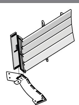
\*Please read **Assembly Tips** before beginning assembly. Fit the Back Brace long edge into the Backs groove track cut out so that the center cut outs on the Back Brace and the Back align. Fit Back & Back Brace ends into the Left Base Sides pocket cut outs. Place Block G into the Back Brace cutout, insert Bolt through Block G into the Base Side and finger tighten.
