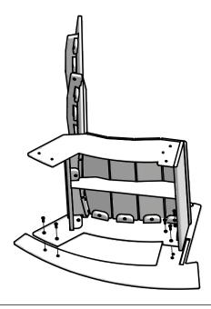
A. Align holes and cut out of the right Leg with the Base Side's holes and Face Plate End. Insert bolts through the Base Side into the right Leg and finger tighten.
