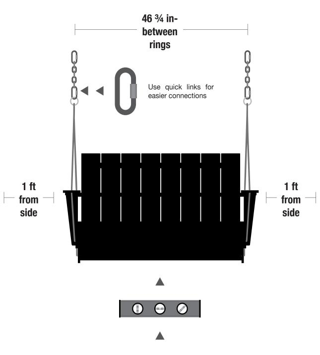
Check that the swing hangs level. Use a level on the swing seat for best measurement.
