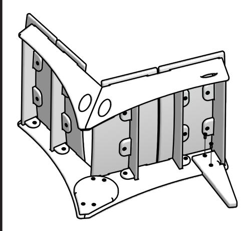
Place Left Leg into Base side by pressing it into the  $\mbox{\rm oval}$  cut.
