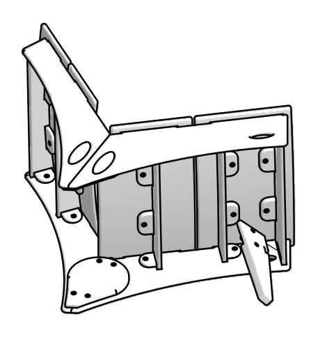
\*Please read **Assembly Tips** before beginning assembly. Set Back and Base on their sides and align as seen above. Fit Left Connection Block with the Back and Base's oval cut outs. Place Bolts through the holes in the Connection Block into the threaded holes of the Back and Base. Finger tighten. Repeat this step for the Right Connection Block then tighten bolts using provided wrench.
