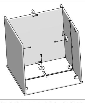
Place G Block's into the Floor's cutouts, insert bolts through the blocks into the Face and Side's threaded holes, and finger tighten.
