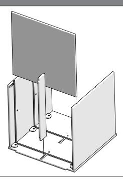
Slide Floor between Side panels by fitting it into the Side's cutouts and sliding into the Face's cutout. The Floor's pocket cutouts should be on the same side as the threaded holes in the Side's and Face. Fit Floor Brace end into the Face's middle cutout.
