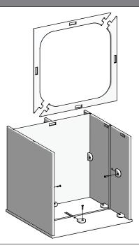
Link Ring Braces together by interlocking the ends together. Fit combined pieces into middle set of cutouts in the Side's and slide down into the Face. The Ring Brace's pocket cutouts should be on the same side as the threaded holes in the Side's and Face.
