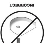
Insert bolts through countersunk hole side of blocks as shown below.
