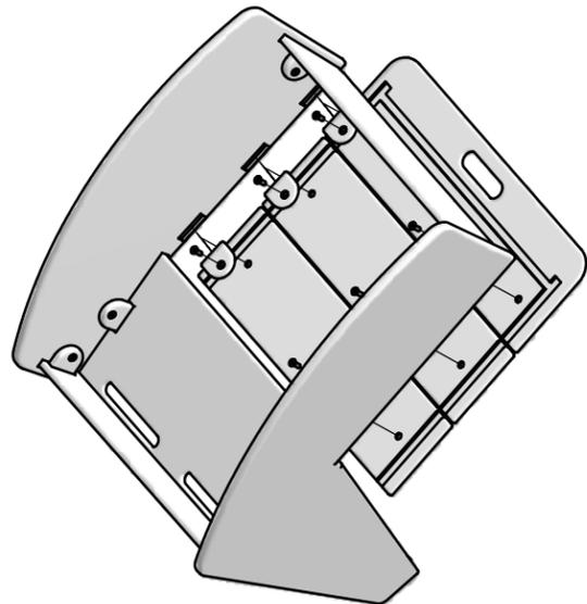
Layout the Seat Set so that the groove track cut outs line up. Place Seat Set individually over assembled chair sides (start with A then B and C) by fitting the groove track cut outs with the Sides and Front Plate. Place G Blocks into the Sides pocket cut outs, insert bolts through the blocks into the Seat Sets threaded holes, and finger tighten.
