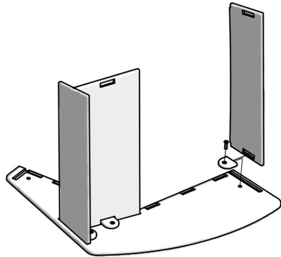
Fit Face Plate short edge into the Left Side's pocket cut out. Place G Block into the Face Plate's pocket cut out, insert a bolt through the block into the Left Side's threaded hole, and finger tighten.
