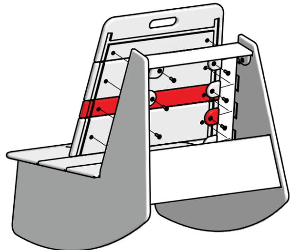
Layout the Back Set so that the groove track cut outs line up. Place Back Set individually over assembled chair sides (start with A then B, C, D) by fitting the groove track cut outs with the Sides and Front Plate. Place G Blocks into the Sides pocket cut outs, insert bolts through the blocks into the Back Sets threaded holes, and finger tighten.
