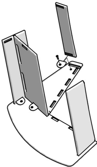
Fit Top Brace edge into Left Side's pocket cut out. Place G Blocks into the Top Brace's pocket cut out, insert a bolt through the block into the Left Side's threaded holes, and finger tighten.
