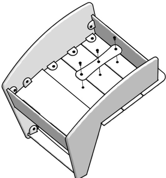
Align Seat Brace holes with the holes of the Seat Set, then insert bolts through the Seat Brace into the Seat Set's threaded holes and finger tighten.
