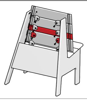
Layout the Back Set so that the groove track cut outs line up. Place Back Set individually over assembled chair sides (start with A then B, C, D) by fitting the groove track cut outs with the Sides and Front Plate. Place G Blocks into the Sides pocket cut outs, insert bolts through the blocks into the Back Sets threaded holes, and finger tighten.
