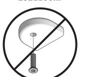
jusert bolts through countersunk hole side of blocks as shown below.
