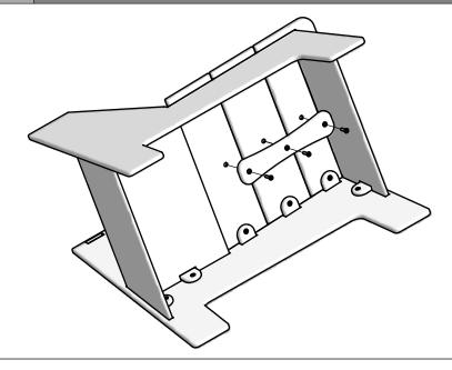
Align Seat Brace holes with the holes of the Seat Set, then insert bolts through the Seat Brace into the Seat Set's threaded holes and finger tighten.
