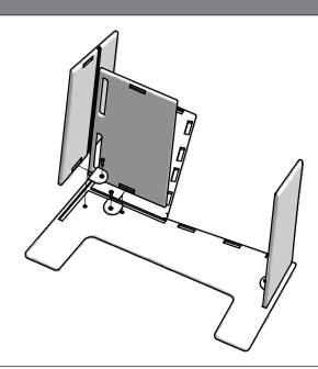
Fit edge of Lower Shelf that has holes through it into the groove track cut out of the Back Plate, and fit both pieces into the groove track cut outs of the Left Side. Place G Blocks into the Lower Shelf and Back Plates pocket cut outs, insert bolts through the blocks into the Left Sides threaded holes, and finger tighten
