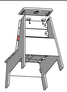
Fit Top Shelf pocket cut outs with top edges of Left & Right Sides (be sure handle is toward back). Place G Blocks into the Sides pocket cut outs, insert bolts through the blocks into the threaded holes of the Top Shelf, and finger tighten.
