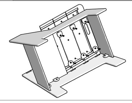
Layout the Seat Set so that the groove track cut outs line up. Place Seat Set individually over assembled chair sides (start with A then B and C) by fitting the groove track cut outs with the Sides and Front Plate. Place G Blocks into the Sides pocket cut outs, insert bolts through the blocks into the Seat Sets threaded holes, and finger tighten.
