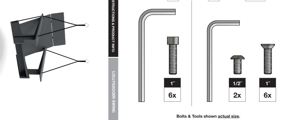
\*\*\* Please double check the bolt size required on each step. Use of wrong bolts will result in damage of product.\*\*\*
