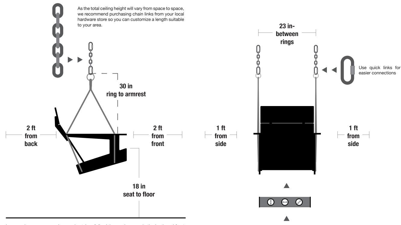
In general, we recommend approximately a 2-ft minimum clearance in the back and front, and a foot on either side. As far as the seat height, we recommend it to be approximately 18" from the ground, but that can be a general approximation, due to each specific user.
