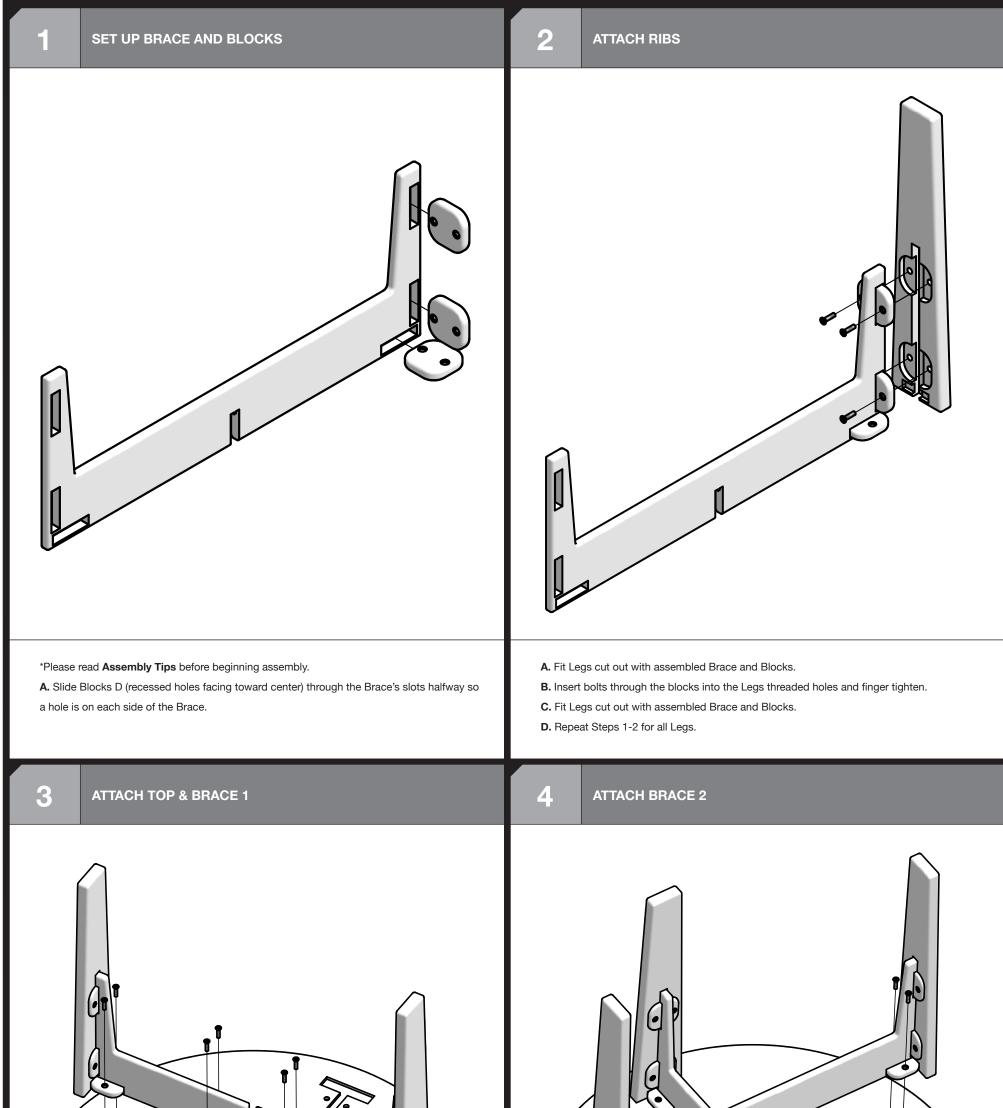
A. Fit Brace 1 with assembled Legs into the Top's track.B. Slide Blocks D through the remaining two slots in Brace 1.C. Attach using bolts.
